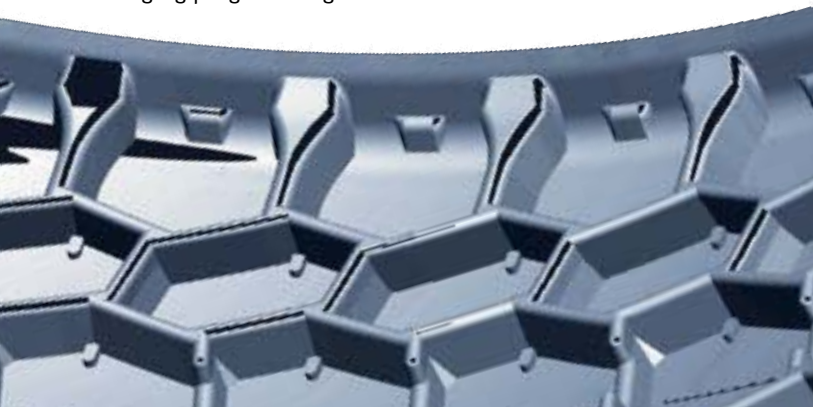
5axis Swarf machining with conical ball mill
