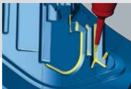
3D-automated rest machining for homogeneous toolpaths
